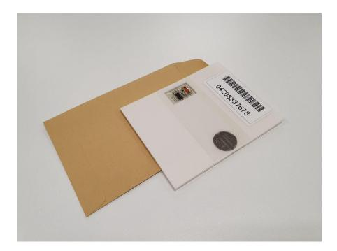
This type of RFID tag is enclosed within the test item in its own envelope.
